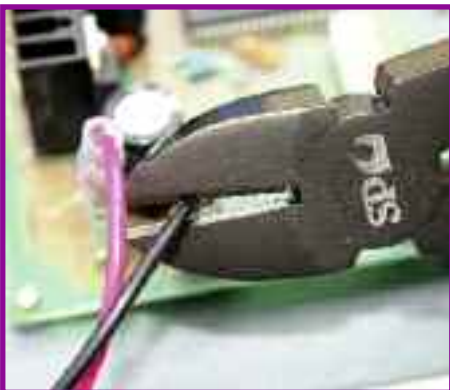
Induction hardened high quality cutting edges
