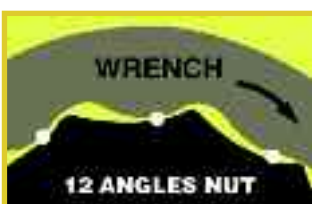
Flat drive technology - maximum contact on flats, not points
