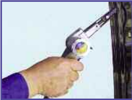
Adjustable belt guide rotates 160 degrees and allows belt replacement in seconds
