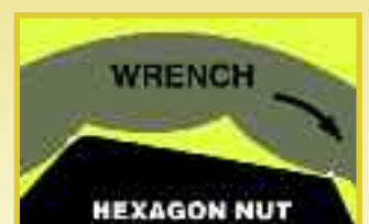
Standard technology - contact at points
