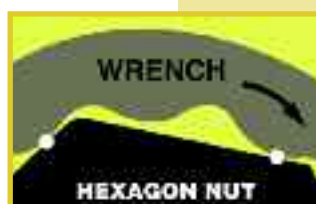
Flat drive technology - maximum contact on flats, not points
